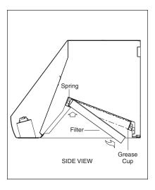
Filter and grease cup installation
